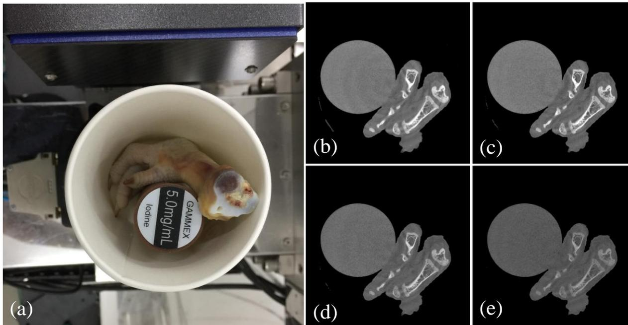
Preclinical experiment. (a) is the preclinical specimen fixed on the spectral CT system. (b)-(e) are FBP reconstruction results from 4 energy bins, where the display window is  $[0 \ 0.5] \text{ cm}^{-1}$
