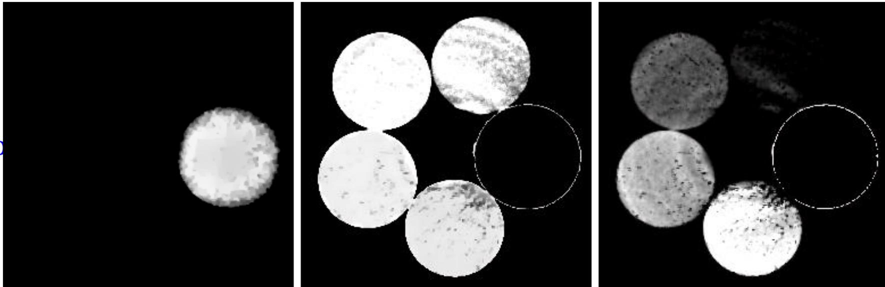
From left to right, the columns represent the decomposition results of aluminum, water and iodine, where the display windows are  $[0.5 \ 1]$ ,  $[0.8 \ 1]$  and  $[0 \ 0.003]$ .
